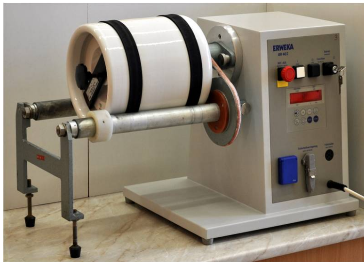
Fig. 20.6. Laboratory scale batch operation ball mill
