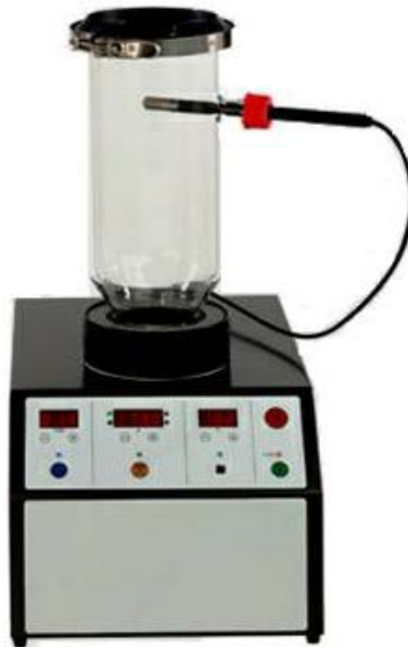
Fig. 19.11. Laboratory scale fluidized bed dryer
