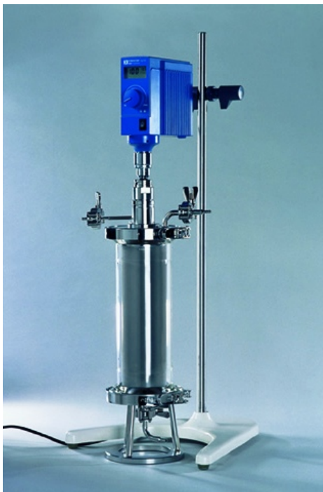
Fig. 17.7. Laboratory filtering centrifuge
