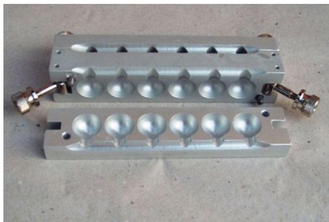
Fig. 13.19. Casting mold for globules
