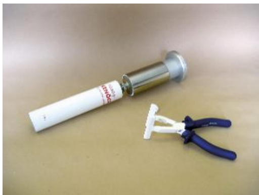
Fig. 13.6. Officinal ointment tube filler and crimping tools
