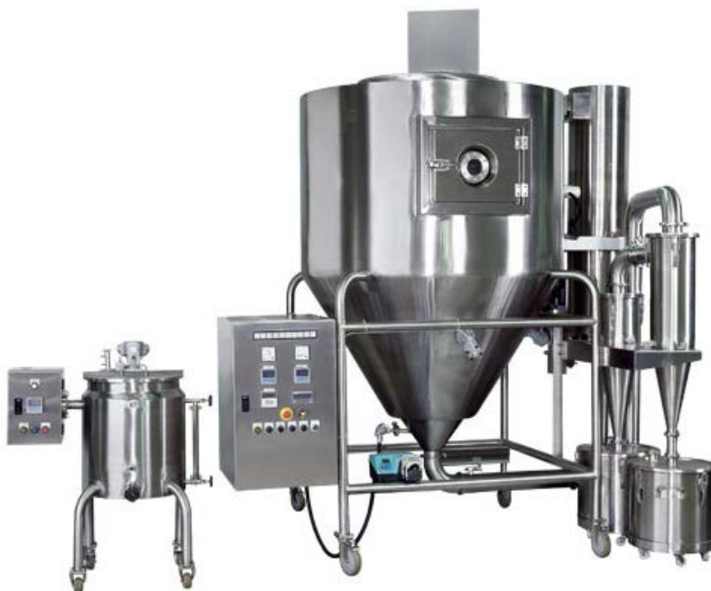
Fig. 27.14. Industrial equipment for-spray freeze-drying
