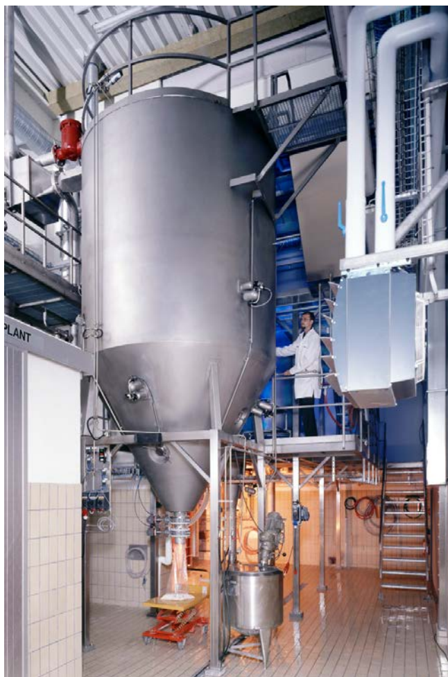
Fig. 19.18. Production scale GEA spray dryer
