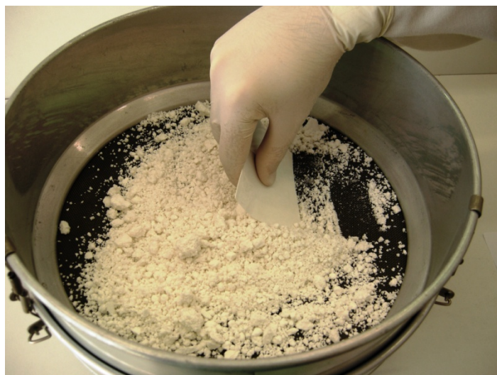
Fig. 23.25. Manual granulation, breaking through a sieve
