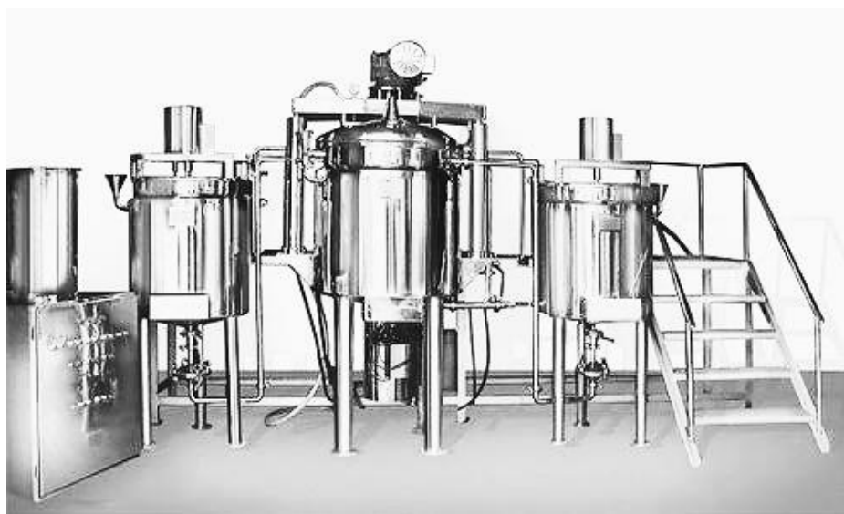
Fig. 13.5. industrial scale ointment production line
