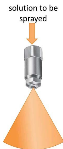
Fig. 19.14. Mechanical spray drying nozzle
