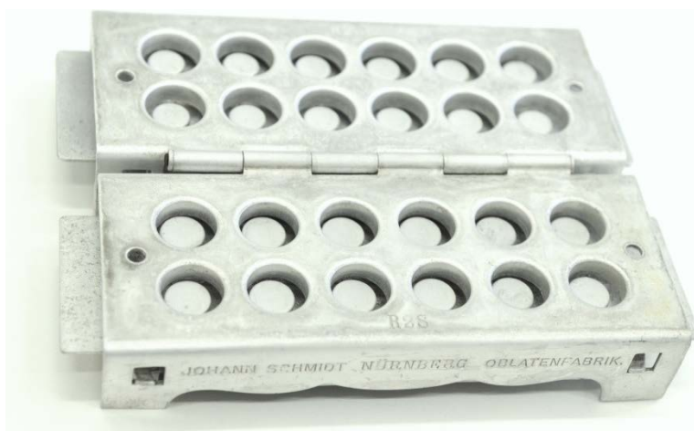
Fig. 25.1. Laboratory wafer capsule filling device
