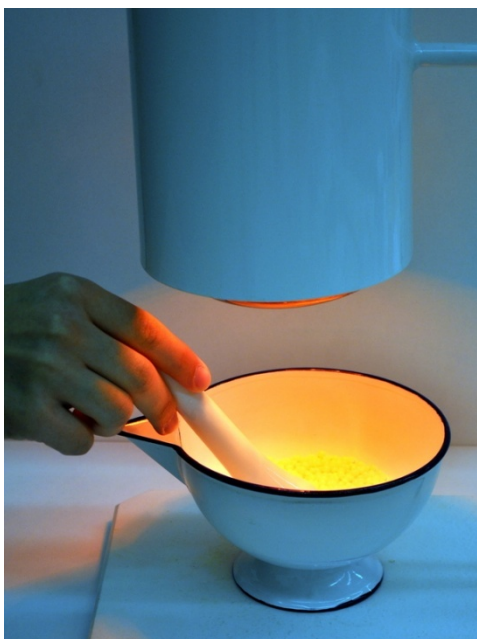
Fig. 7.3. Melting of ointment basis by infra lamp
