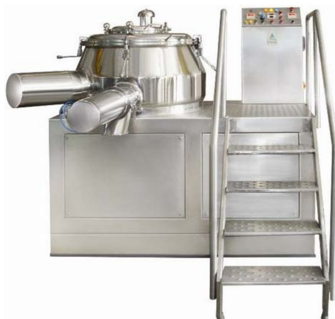
Fig. 23.30. Industrial Diosna-type high-shear granulator with control unit
