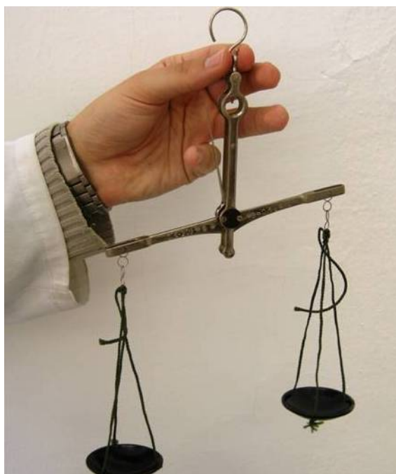
Fig. 6.2. The pharmaceutical hand-scale
