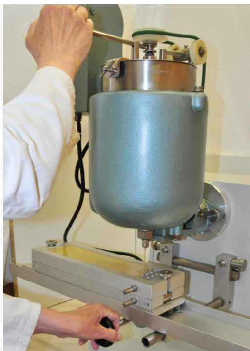
Fig. 13.14. Laboratory and medium-scale manufacturing of suppositories with an Erweka device
