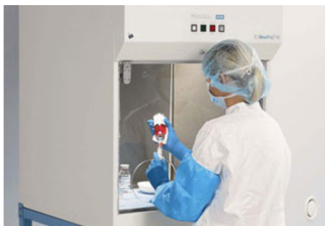
Fig. 28.3. LAF device for preparing cytostatic compounds
