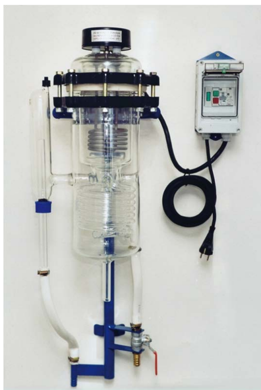
Fig. 9.10. Water distillation device
